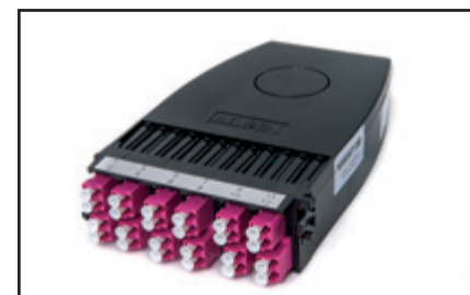
FC4U12LDMF, FX Ultra Cassette, OM4, 12 ports, MPO-12 (male), LC Duplex, Type-A, Erika Violet adapters
